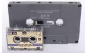
Fig. 2.1. A compact cassette and a (smaller) microcassette
