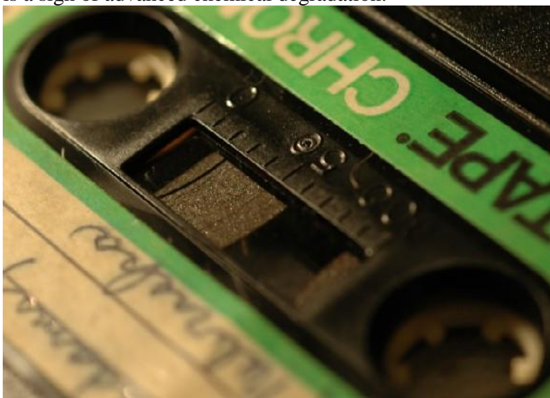
Fig. 2. 4 Crystal deposits on a sound cassette
